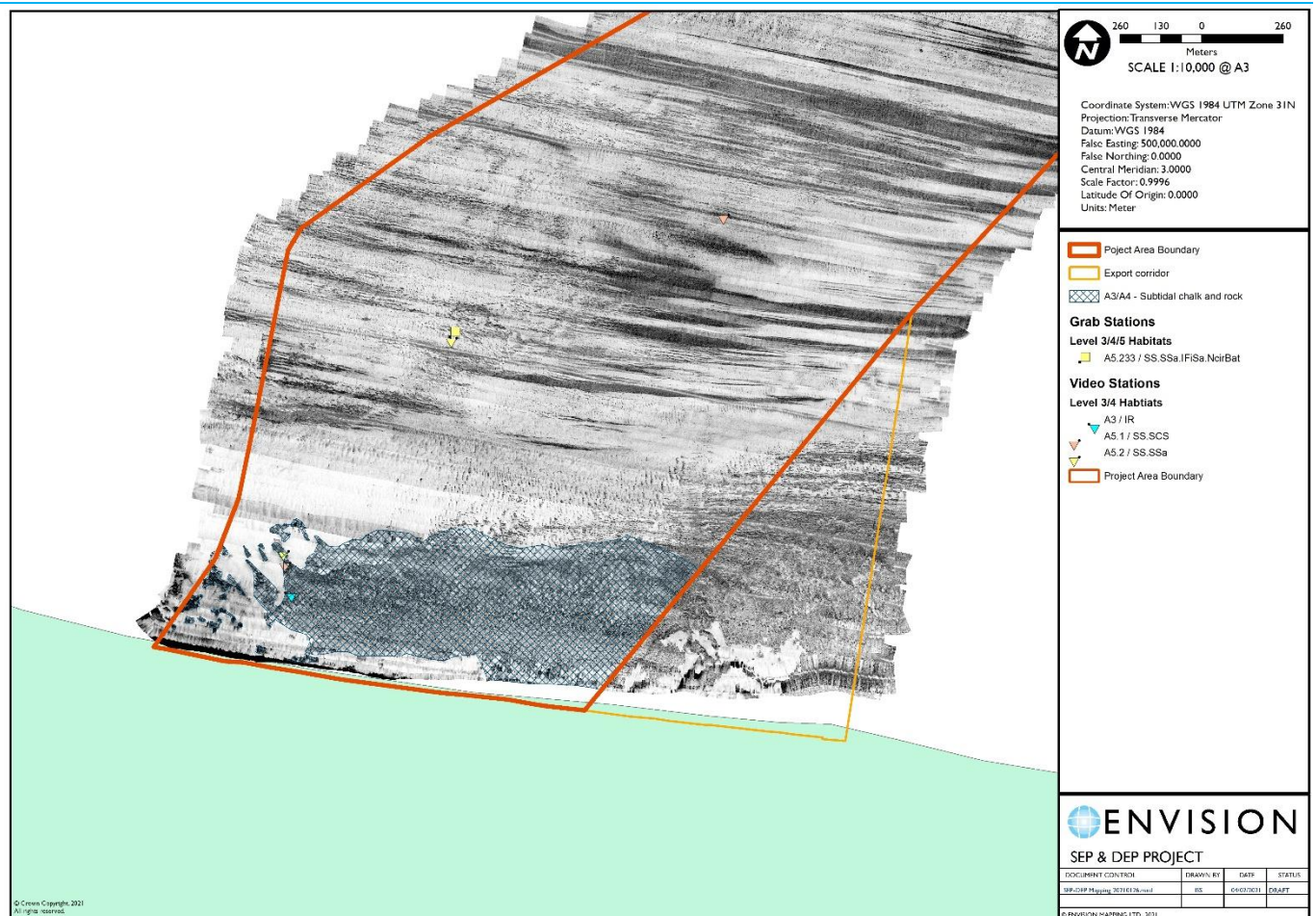
Figure 15. Extent of subtidal chalk and rock features digitised using sidescan and bathymetric data for the inshore section of the export cable corridor for the SEP-DEP project
